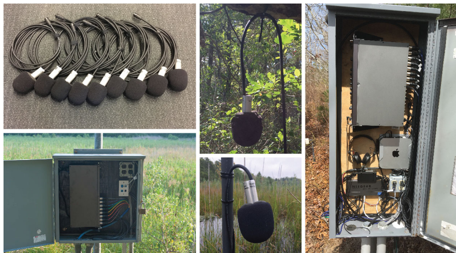
Fig. 3: Fixed audio capture at Tidmarsh: 24 microphones are connected to a 32-channel mixer and audio interface, whose output is compressed into a Ogg/Opus stream.
