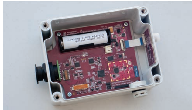
Figure 3. The second-generation hardware inside the waterproof enclosure.
